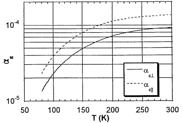
Figure 2: Thermal coefficients of permittivity for sapphire evaluated from measurements of whispering gallery mode resonant frequencies versus temperature.
