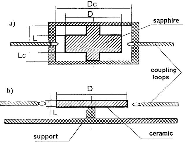
Figure 1: Whispering-gallery mode resonant structures used in laboratory experiments: (a) sapphire resonator, (b) dielectric ceramic resonator.
